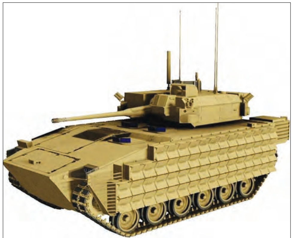
U.S. Army Acquisition Support Center drawing The optionally manned fighting vehicle prototype shown here will replace the U.S. Army's Bradley fighting vehicle.
